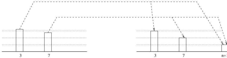
Figure 11.2: The general-to-grained filter (as applied to part of the fixed distribution q that satisfies q(3) = 3.2/6n and q(7) = 2.8/6n ). The dotted lines indicate multiples of \gamma/n , for \gamma = 1/6 .
